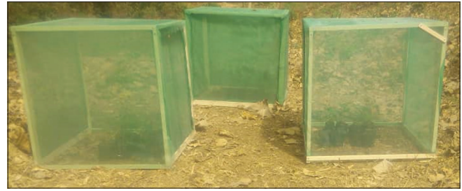
Figure 1: The constructed cages made of aluminum covered on all sides with one (right), two (left), and three layers (middle)
