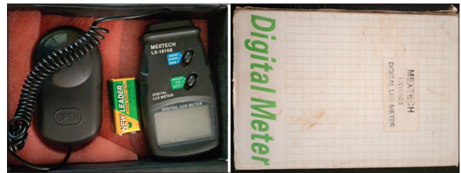
Figure 2: Light meter (Digital Lux Meter Model LX-101, Taiwan) used in monitoring the light intensity within and outside the cage
