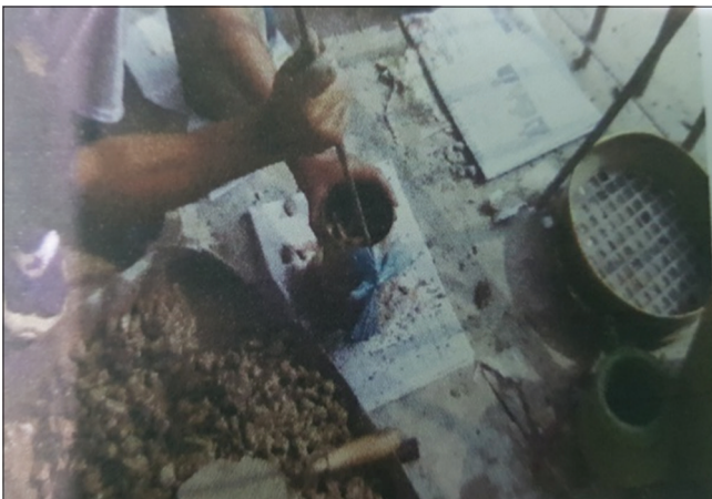
Figure 3: Tamping of aggregate after mixing fibers
