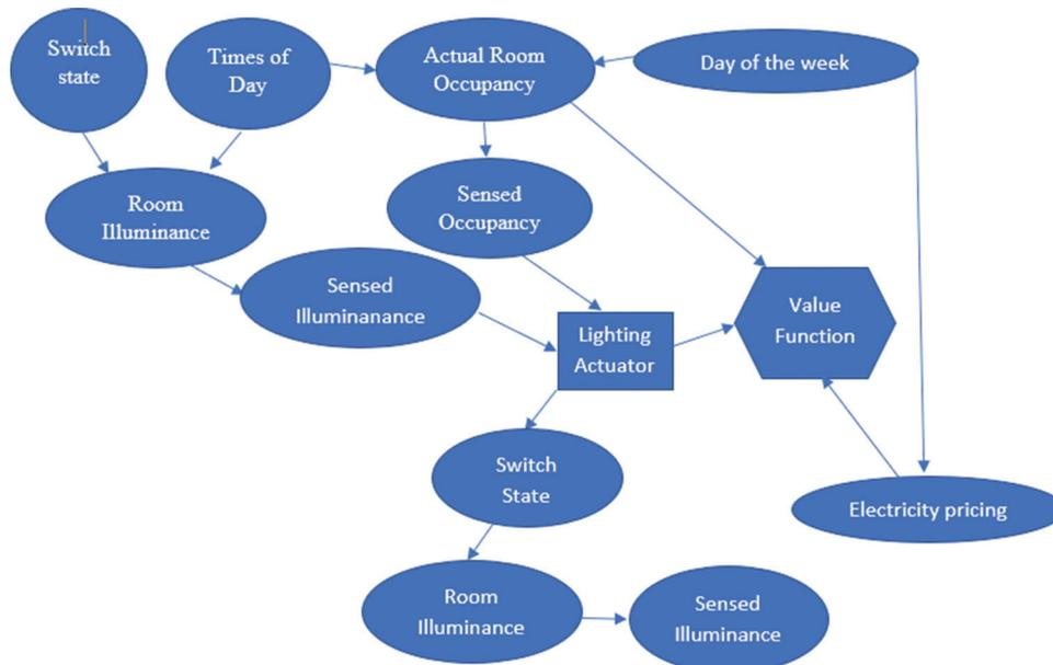
**Figure 3:** Influence diagram for smart lighting control
