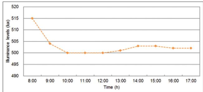
Figure 14: Average illuminance levels under the proposed RBFN controller
