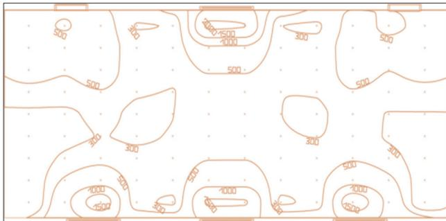
**Figure 15:** Isoline from both daylight and artificial light at time 13:00
