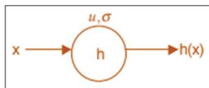
Figure 6: A simple radial basis neuron
