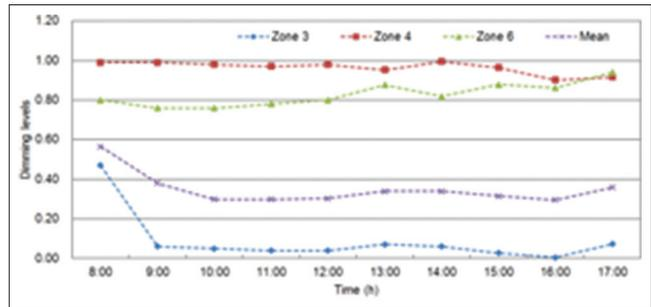
Figure 13: Dimming levels of luminaires results for selected zones and their mean
